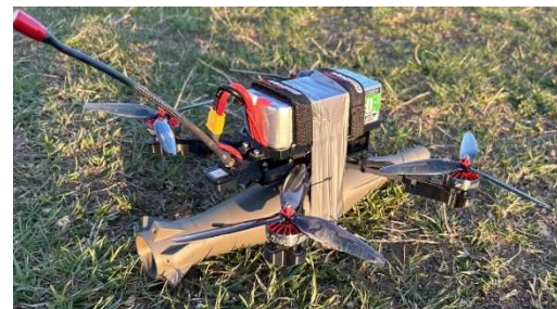
Fig. 1 FPV UAS with explosive device Source: author.
