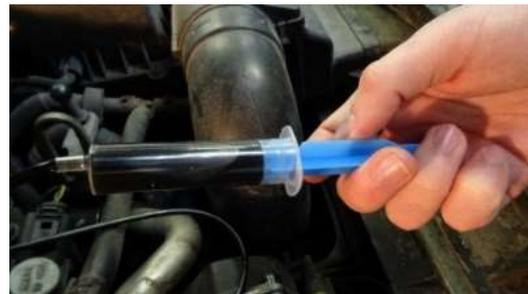
**Fig. 5** Sampling with syringe
