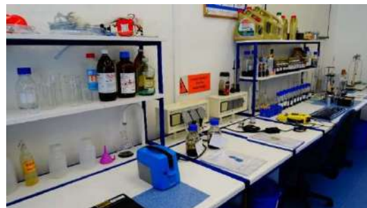
Fig. 2 Tribodiagnostic Laboratory - SpectroVisc Q3050-blue, Spectro Q1000 Fluidscan-yellow Source: authors.
