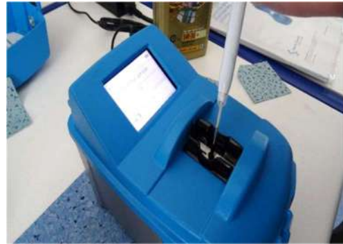
Fig. 16 Application of oil sample Source: authors.
