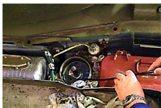
Fig. 7 Oil sampling from MAF cleaner Source: authors.
