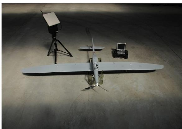
**Fig. 3** The Elements of Fly Eye
