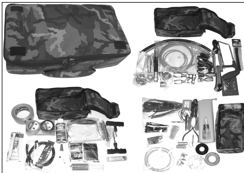
Fig. 1 Battle damage repair kit for repair of land vehicle IVECO [own source]
