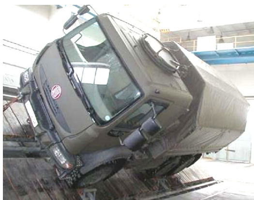
Fig. 5 Example of centre of gravity measuring
