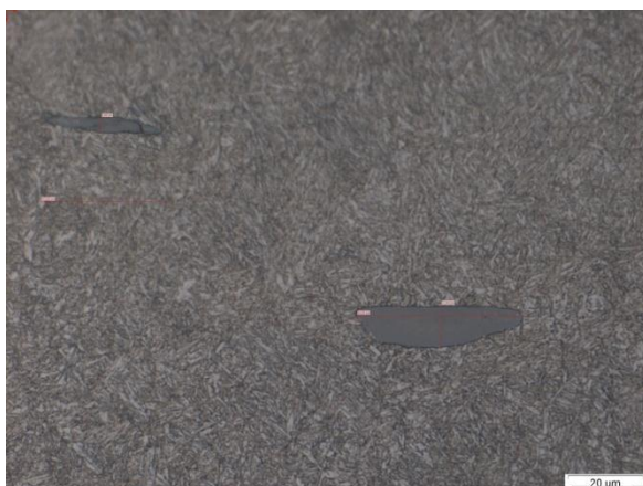
Fig. 3 Sulfide inclusions of enormous size
