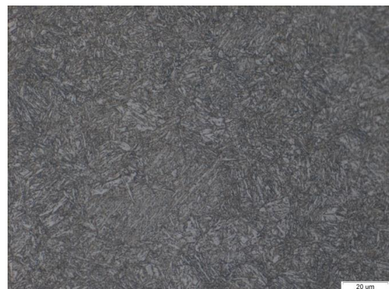
Fig. 6 Microstructure for Charpy impact test perpendicular to the longitudinal axis of the main tank gun (sample No 1.)
