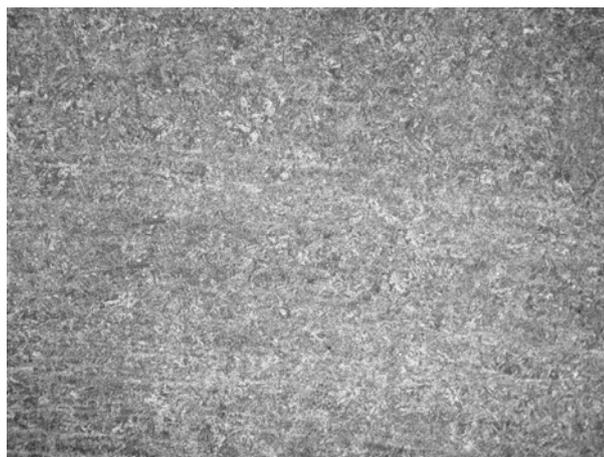
Fig. 4 Microstructure of base material (ARMOX 500), 500x
