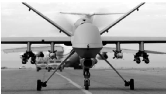
Fig. 5 MQ-9 Reaper with mixed armament
