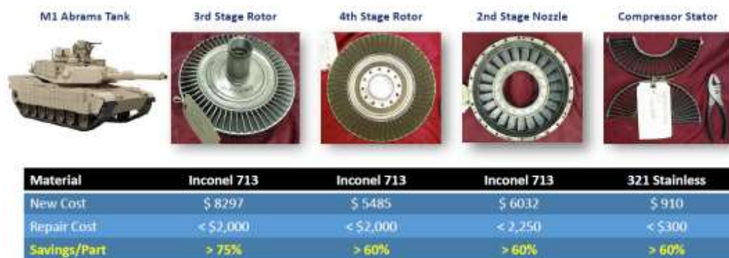
Figure 4 Example: US Army repair of components from Honeywell AGT 1500 gas turbine engine
